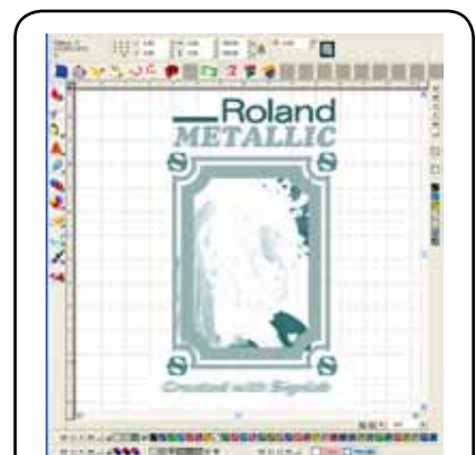
Fig. 41 - Use [Ctrl + click] to hide the Color sheet layer, so that the metallic ink objects can be inspected.
