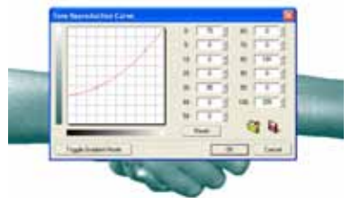
Fig. 7 - The Tone Reproduction Curve is used to adjust the quantity of ink that is laid down in the shadows, midtones and highlights.
