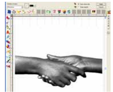
Fig. 6 - Converting the bitmap to multitone allows us to use metallic inks instead of CMYK.
