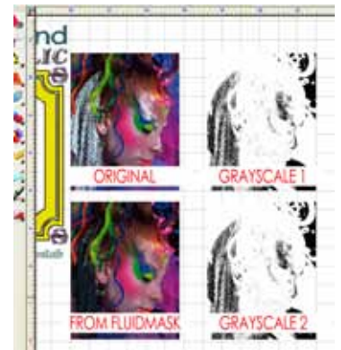
Fig. 37 - After duplicating the grayscale bitmap, we need to invert one and combine it with the original.
