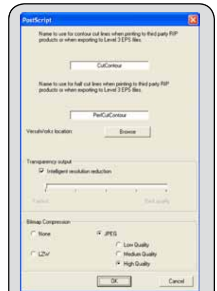
Fig. 1 - When printing a job, a PostScript file is sent to the VersaWorks RIP software. To ensure that VersaWorks recognizes cut paths, confirm the name used to identify cut paths in the PostScript file.
