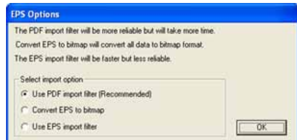
Fig. 5 - When sending EPS data, SignLab will provide further options as to how the data should be interpreted. For best results, import the data as PDF.
